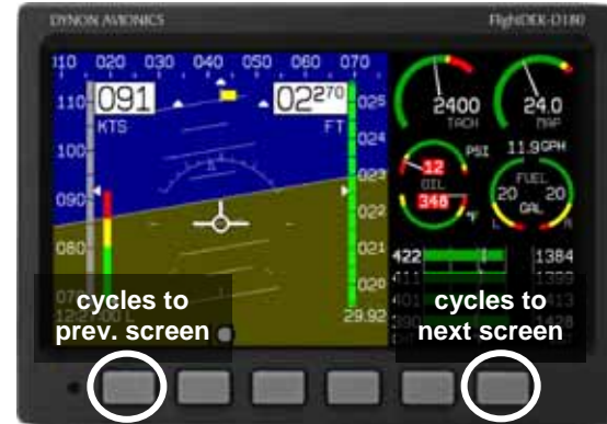
Buttons one and six cycle to the previous and next screens, respectively.
